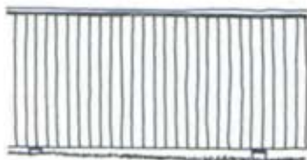
▪ Vertical board with top rail
